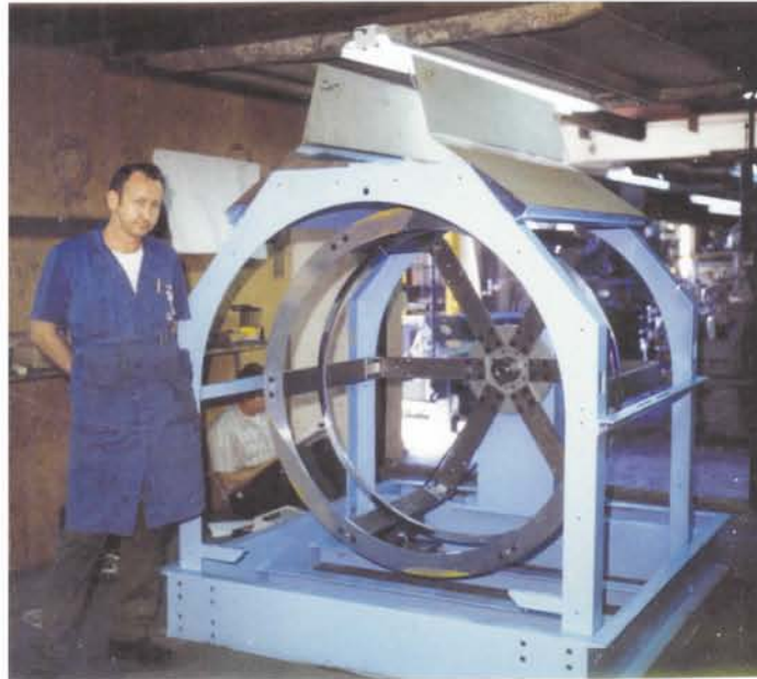
Donald Holt, Founder (1934-2004) Assembling a Beltwinder for artificial kidney manufacturing, 1970.
